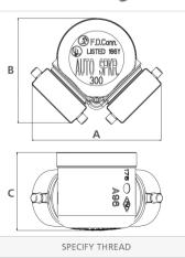
Exposed auxiliary inlet connection with 500 G.P.M. inlet capacity to supplement fire protection water supply. Exposed design provides an economical method of satisfying Fire Dept. inlet requirements.
