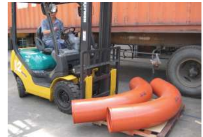
12" 3D 90° elbows ready for shipment
