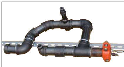
Burst pressure testing of DI threaded fittings (2’)
