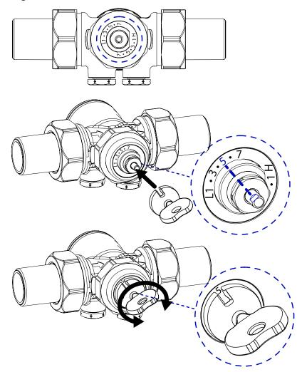
The BS9250015/20/25 valves are equipped with a double regulation scale of the flow rate:
