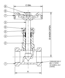
PRESSURE RATING: PN32 TEMPERATURE OPERATING RANGE: 32 Bar at -10 to 100°C 14 Bar at 198°C END CONNECTION: Threaded BS 21 or ANSI B1.20.1 **SPECIFICATION:** Valve are manufactured in accordance with BS 5154 PN32 for Series B ratings. The needle disk is an integral part of the stem, and body seat is integral.
