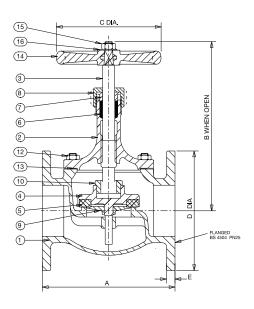
**SPECIFICATION:** Valves are manufactured in accordance with BS 5154 PN25 for series B ratings with 'long' face-to-face. Design incorporates disc holder which on sizes 15 to 50 slips on to stem and on sizes 65 and 80 is retained by a threaded ring. Body seat is integeral of the semi-crown type. Sizes 15 to 50 have union bonnet; sizes 65 and 80 have a bolted bonnet.
