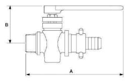
PRESSURE RATING: PN10 TEMPERATURE OPERATING RANGE: -10 to 110°C UK END CONNECTION: Not Specified OPERATOR: Lever Operated
