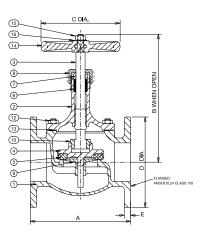
PRESSURE RATING: Class 150 TEMPERATURE OPERATING RANGE: -10 to 186°C UK END CONNECTION: Not Specified US END CONNECTION: Flanged Class 150 OPERATOR: Handwheel AVAILABLE OPTOINS: Flanges Undrilled. P150 Locking Device
