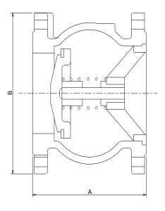
PRESSURE / TEMPERATURE RATING: 16 bar from -10 to 120°C (WRAS to 85°C) SPECIFICATION: Flanged to BS EN 1092-2 PN16.
