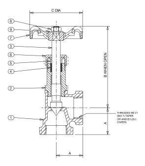
PRESSURE RATING: PN32 TEMPERATURE OPERATING RANGE: 32 Bar at -10 to 100°C 14 Bar at 198°C END CONNECTION: Threaded BS 21 or ANSI B1.20.1
